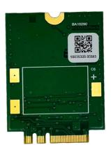
High precision location coordinates are easy to inject into your system with this small M.2 form-factor RTK GNSS receiver. For fast time to market and future-proofing your GNSS solution, all that is needed is an "A" or "E" key M.2 connector slot. When paired with a multi-band antenna, ~2 centimeter range positioning is achievable.
