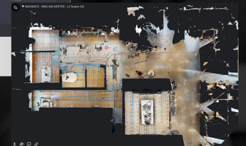
3D camera image of part of a renovation job, used to create a 3D model so the offices could be in use while the clients planned the renovation.
