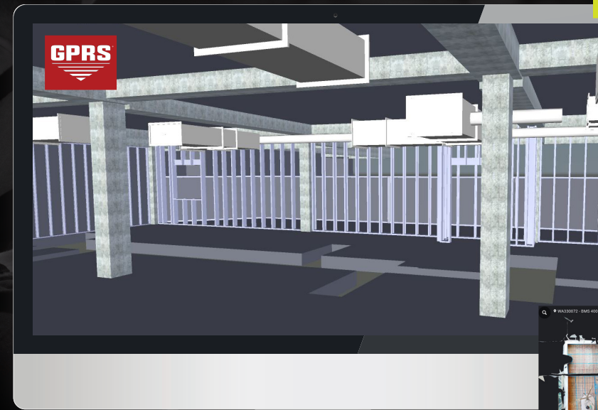
Image from a Revit 3D BIM model of a college lab in Tucson, AZ. 97 scans were completed in one day to build this model that is accurate to within millimeters.
