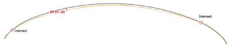
Plan View: SCREEN "A" TOP EDGE Major deviations can be seen on the top edge of the screen.
