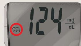
After marking the test result with the appropriate meal marker, remove the test strip to turn the meter off and discard the used test strip.
