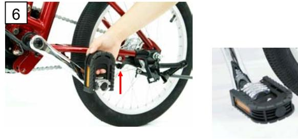
Pull the trigger of the pedal and unfold the pedal simultaneously. Repeat the same steps on the other side of the pedal.
