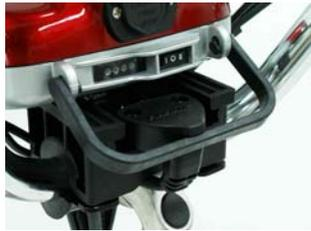
2. Switch the key to horizontal (flat) position. Depress the key to release the lock and use the other hand to push the battery case out from the battery holder.
