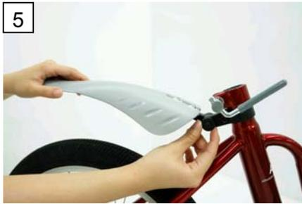
Adjust the tighten knob to fasten the mudguard.
