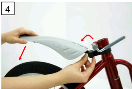
Lower the mudguard by loosening the tighten knob.
