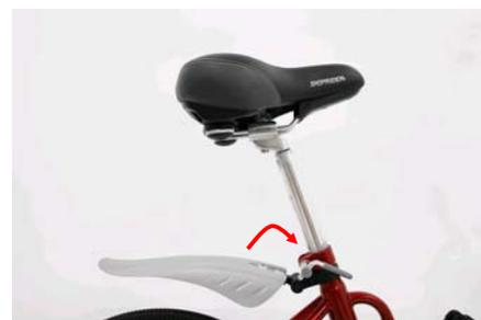
4. Tighten the clamp lever.
