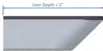
User Seat Depth PLUS 2" Foam Extended Out Front
