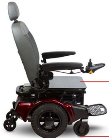
STFH is measured from top of seat pan to floor.
