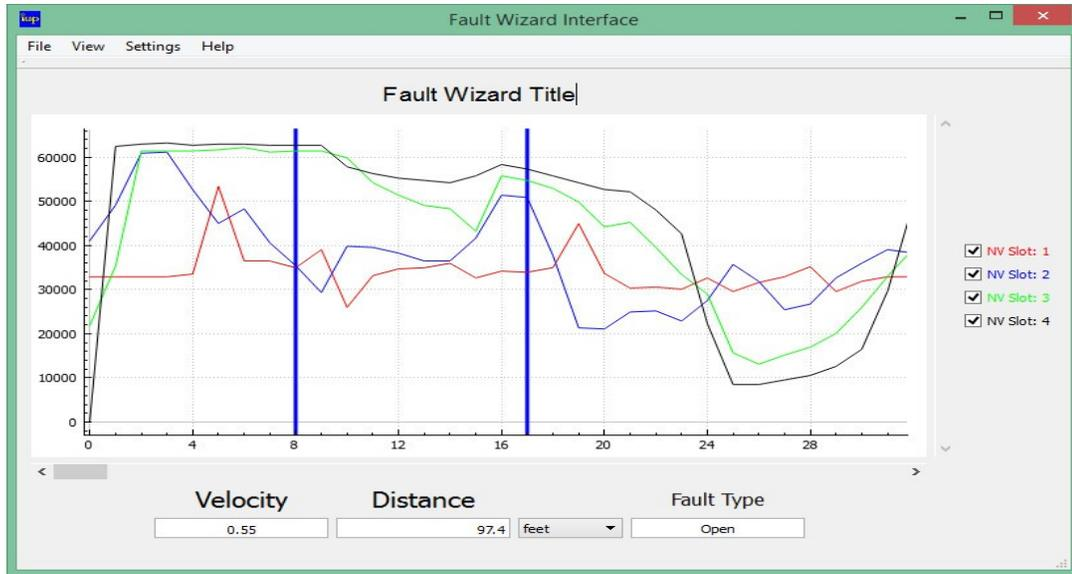
We want to remove the second (blue) waveform from the graph above so, first we'll need to left-click on the waveform to highlight it. Shown below is the highlighted blue waveform.
