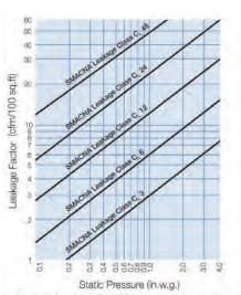
This chart is based on SMACNA HVAC Air Duct Leakage Test Manual, 1985 Edition found in Figure 4-1 under "Duct Leakage Classification".
