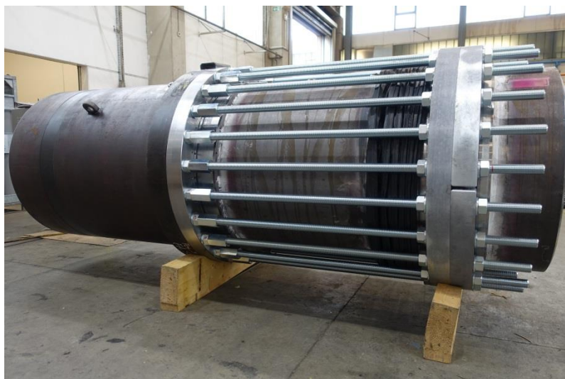
Fig. 1: Expansion joint DN1000 / PN84 during mounting and preparation for the hydrostatic strength test in the factory
