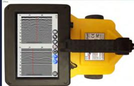
Simulated Radargram screen showing scan line result
