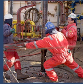
Breaking Out Drill Pipe
