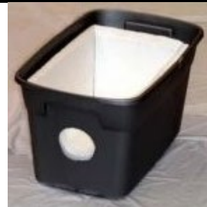
Insert Styrofoam cooler and cut hole to match bin's hole
