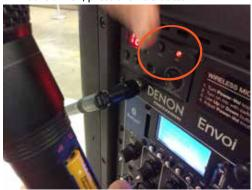
7) The IR light will flash momentarily & turn off. The RF light will light up, indicating the mic and receiver are in-sync.
