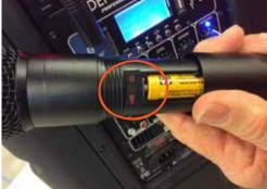
Point the IR Symbol on the transmitter (mic) toward the IR Symbol on the receiver — it's important for the 2 Symbols to "see" each other. Then, press the ASC button.
