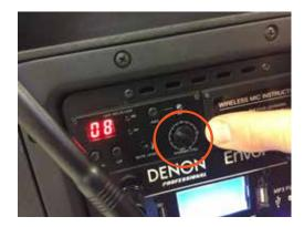
3) Turn on the RF Transmitter (on the bottom of the mic). As you test the microphone, adjust volume of the speaker.
