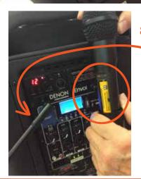
Make sure to close the battery compartment of the RF transmitter the mic). And be sure to raise/extend the antenna.
