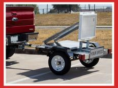
Easy to tow trailer uses a  $1^{7}/_{8}$ " ball hitch. Multiple trailers can be carried on a larger flatbed if needed.
