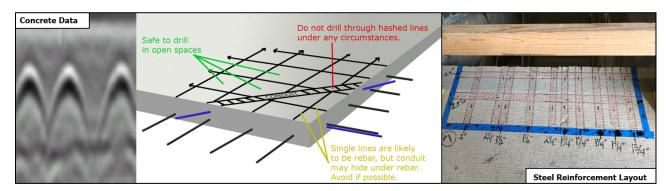
Additional to GPR being used to image steel reinforcement in the slab, *SIM* also calls for a passive sweep of the pipe locator/EM receiver to confirm the area has no energized conduits. GPR is capable of imaging a plastic pipe in concrete but cannot determine if the conduit is energized.
