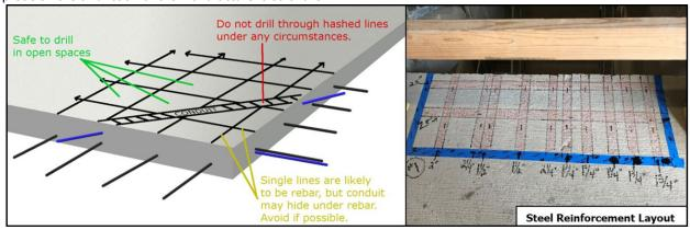
In addition to GPR being used to image steel reinforcement in the slab, *SIM* also calls for a passive sweep of the pipe locator/EM receiver to confirm the area has no energized conduits. GPR is capable of imaging a plastic pipe in concrete but cannot determine if the conduit is energized.
