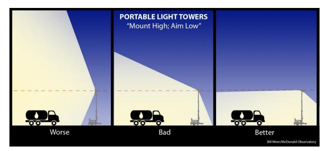
Vehicle-mounted lights or portable light towers are preferred over permanently mounted lighting for nighttime maintenance activities. If possible, such lighting should be equipped with hoods or louvers and be aimed toward the ground to avoid causing glare and skyglow.
